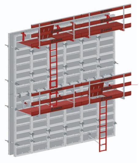
The concreting platform "L" can be attached either to the top of the formwork or to the function profile of the formwork. The assembly adapter for concreting platform "L" is required for this.
